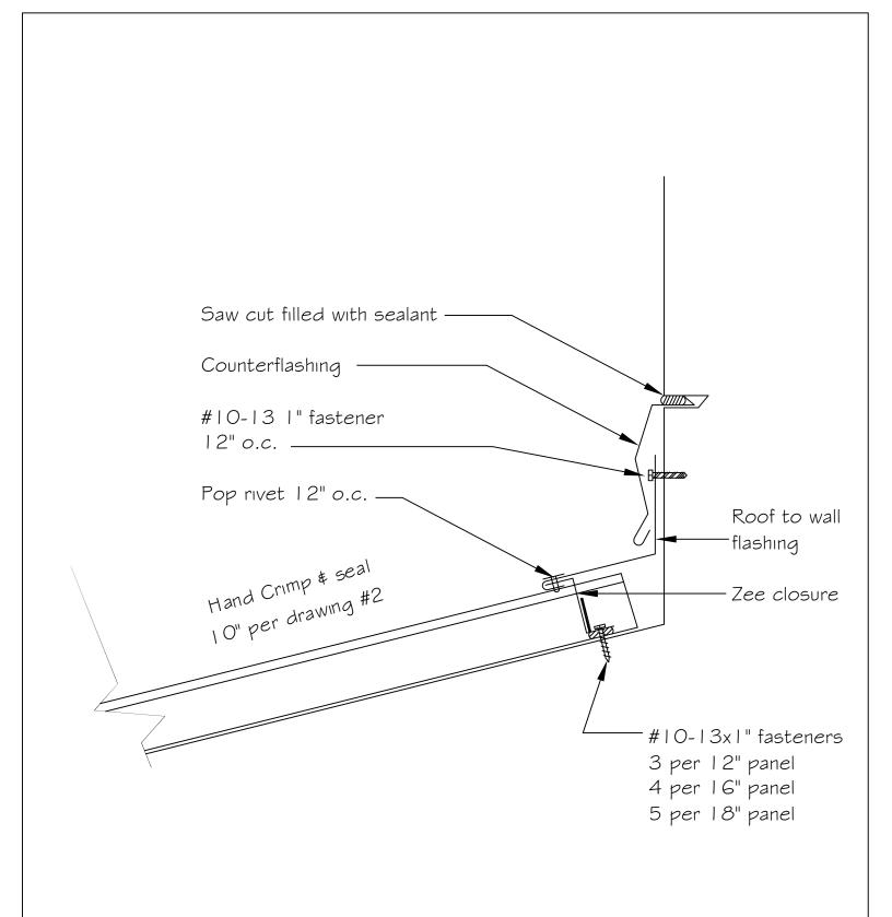
DETAIL: Roof to Wall flashing
