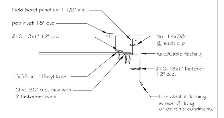
DETAIL: Rake/Gable Flashing
