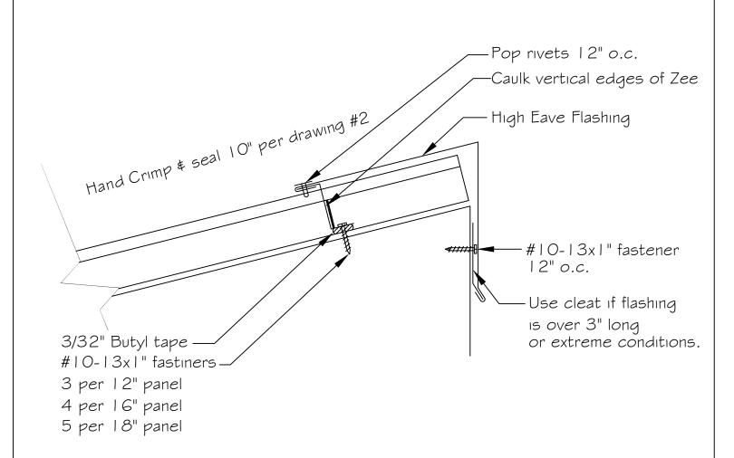
DETAIL: High Eave Flashing
